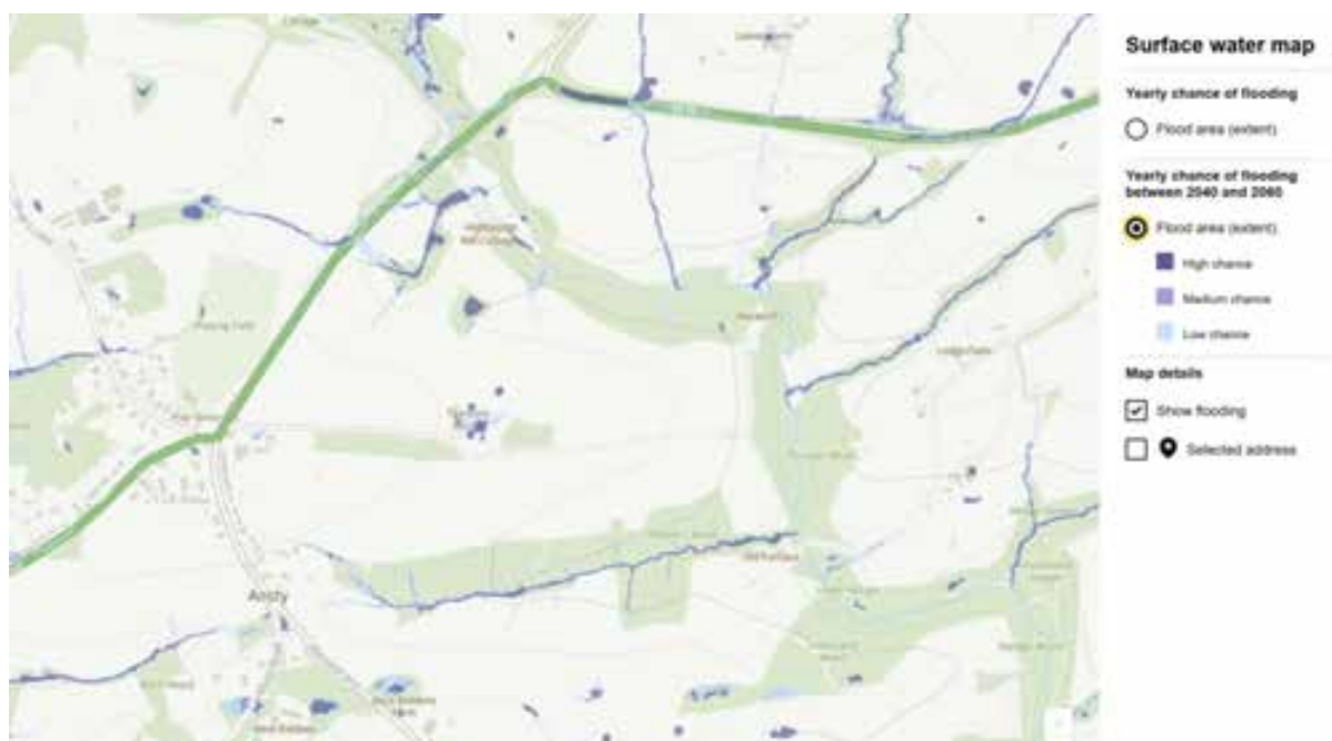
Figure 4-3 Surface water flood risk zones (2040 to 2060 epoch)
