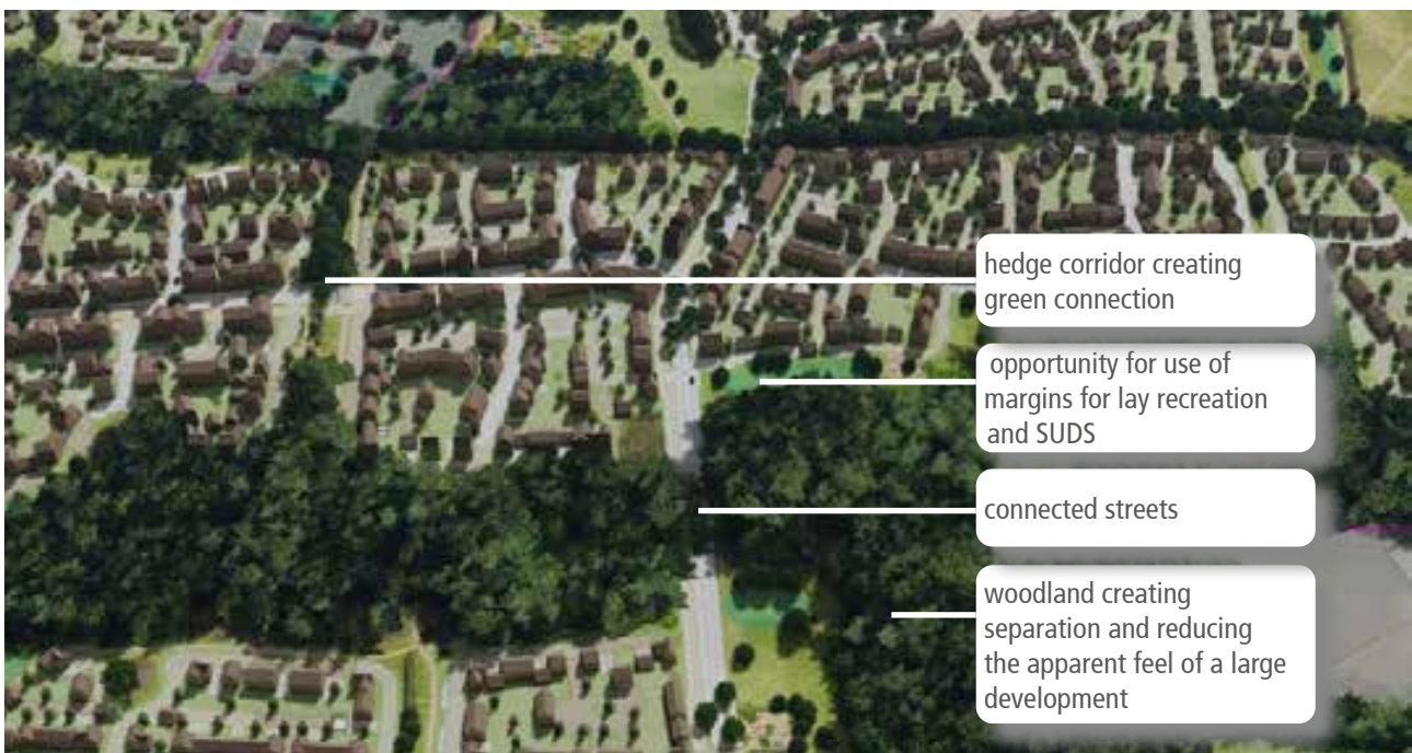
Figure 22. Aerial visualisation of the masterplan (Code page 101) showing parcels separated by woodland blocks
