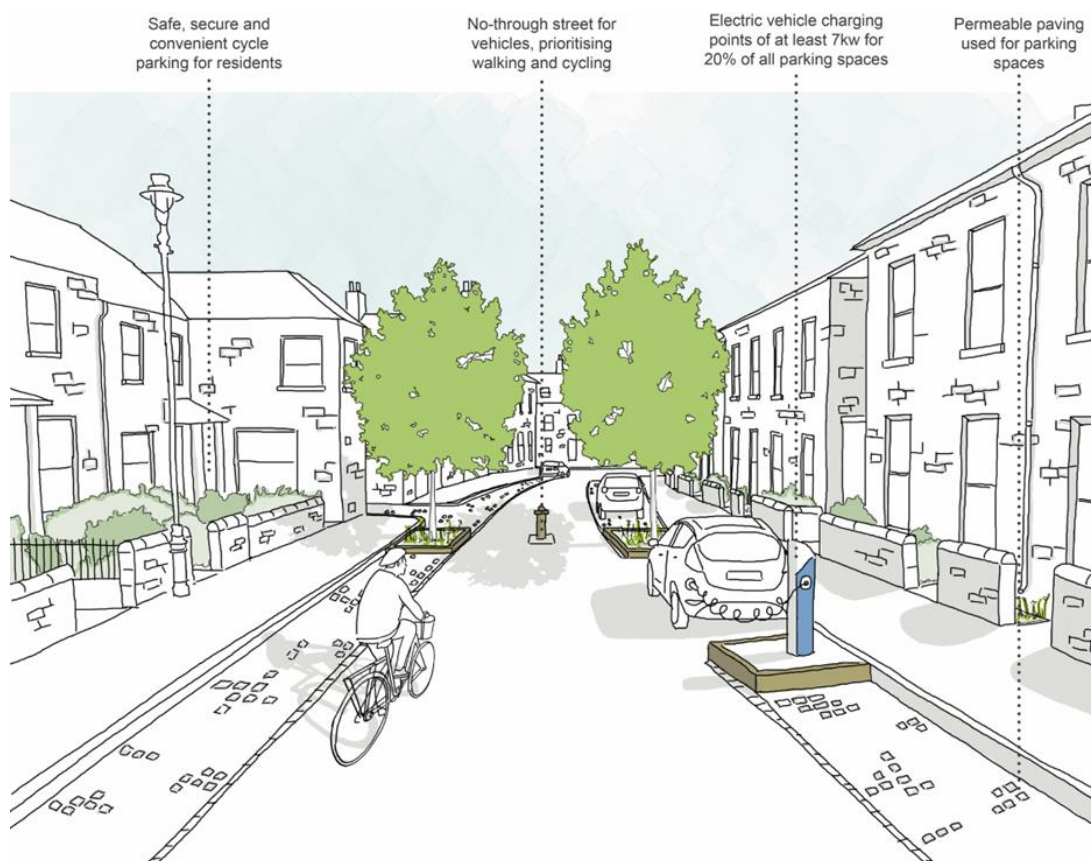
Figure 9. Example of a street which incorporates good design features, including EV charging points
