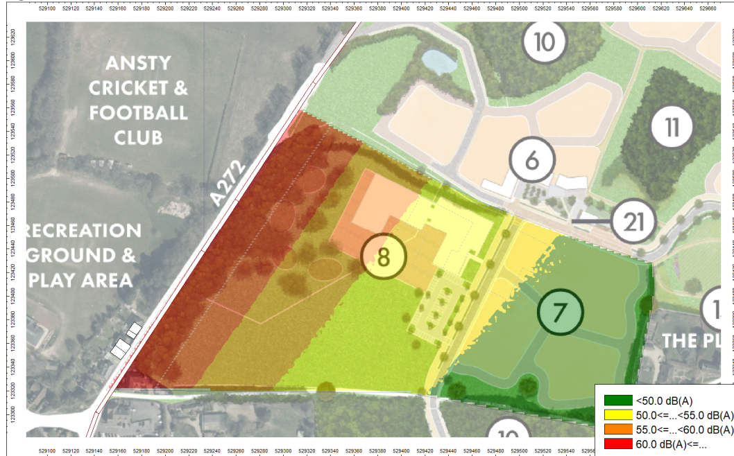
Figure 5.1: Calibrated noise contours (1.5 m AGL) – baseline scenario
