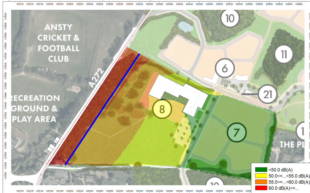
Figure 5.2: Noise contours showing effect of 2m high fence (1.5 m AGL)
