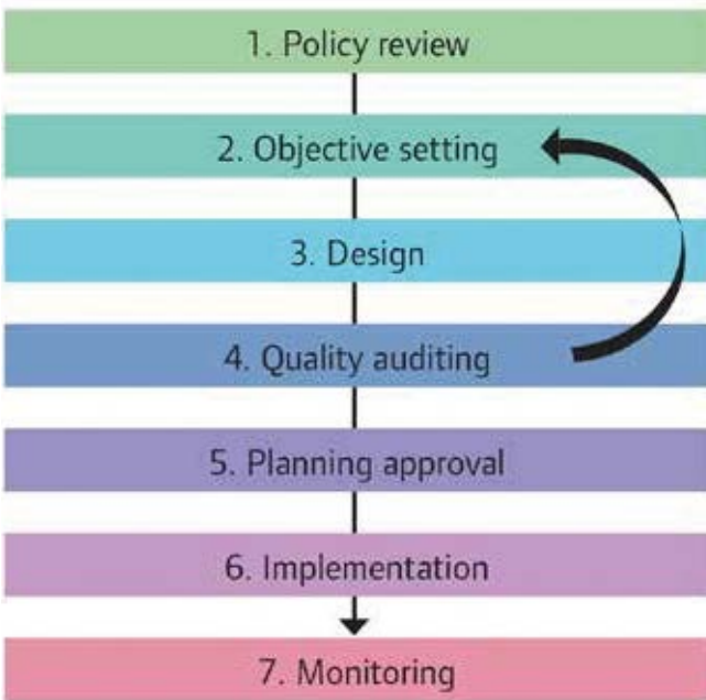
Figure 14.9: Highways, overall improvements process
