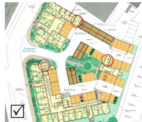
The bin stores serving this East Grinstead block of flats are discretely integrated within the envelope of the building and around the rear courtyard where they avoid deadening the street frontage. They are also well positioned for ease of collection while providing sufficient separation from the adjacent flats to avoid causing undue nuisance
