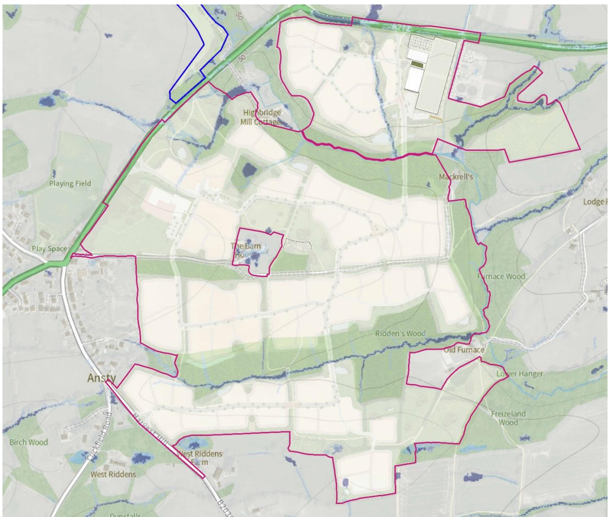
Figure 1: Gov.uk Flood map for planning overlaid with the proposal site red line boundary and illustrative site layout
