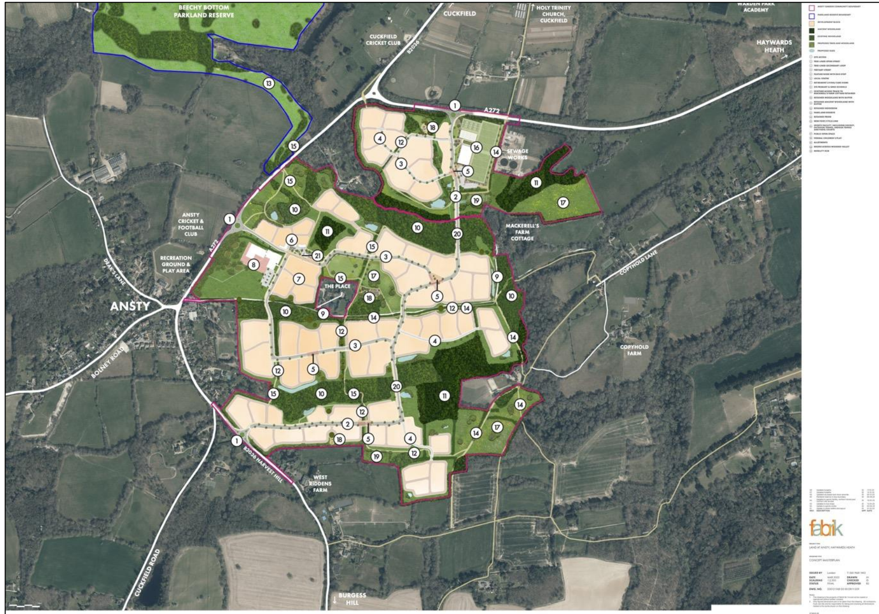
Figure 2. A proposed concept masterplan layout for the development at Land East of Ansty produced by Fabrik, dated 17.10.23 (dwg no. D3012-FAB-00-XX-DR-Y-009-08).
