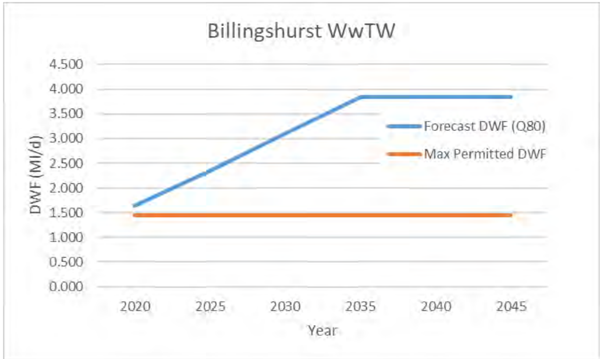
Figure 13.1 Flow Capacity Assessment for Billingshurst
