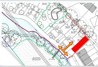
Site office and welfare cabins shall be positioned to the west side of the site entrance by the hammerhead; the pedestrian pathway separating personnel from moving vehicles and plant. The hammerhead shall be fenced off sign road pins and orange fencing to prevent pedestrians entering the turning point.
