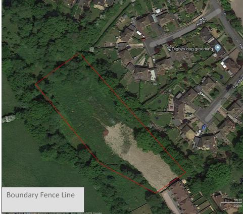
The remainder of the boundaries shall be erected with Heras fencing, double clipped and footed to prevent unauthorised persons entering site. The principal contractor's name board shall be prominently displayed on the boundary fence and hoarding.
