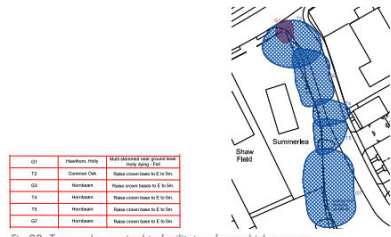
Fig 28: Tree works required to facilitate refuse vehicle access.
