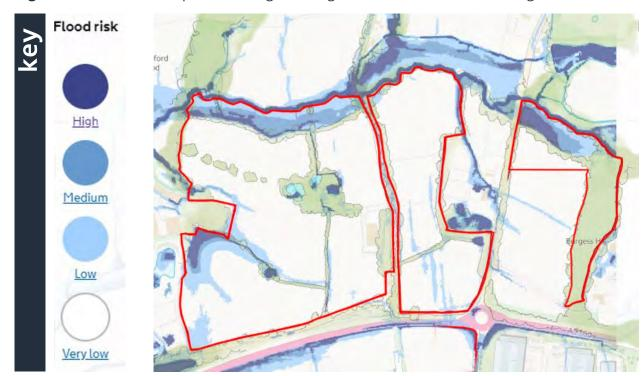
**Fig 7.2** - EA Surface water flooding map, showing areas of ponding/streaming to be incorporated into the development
