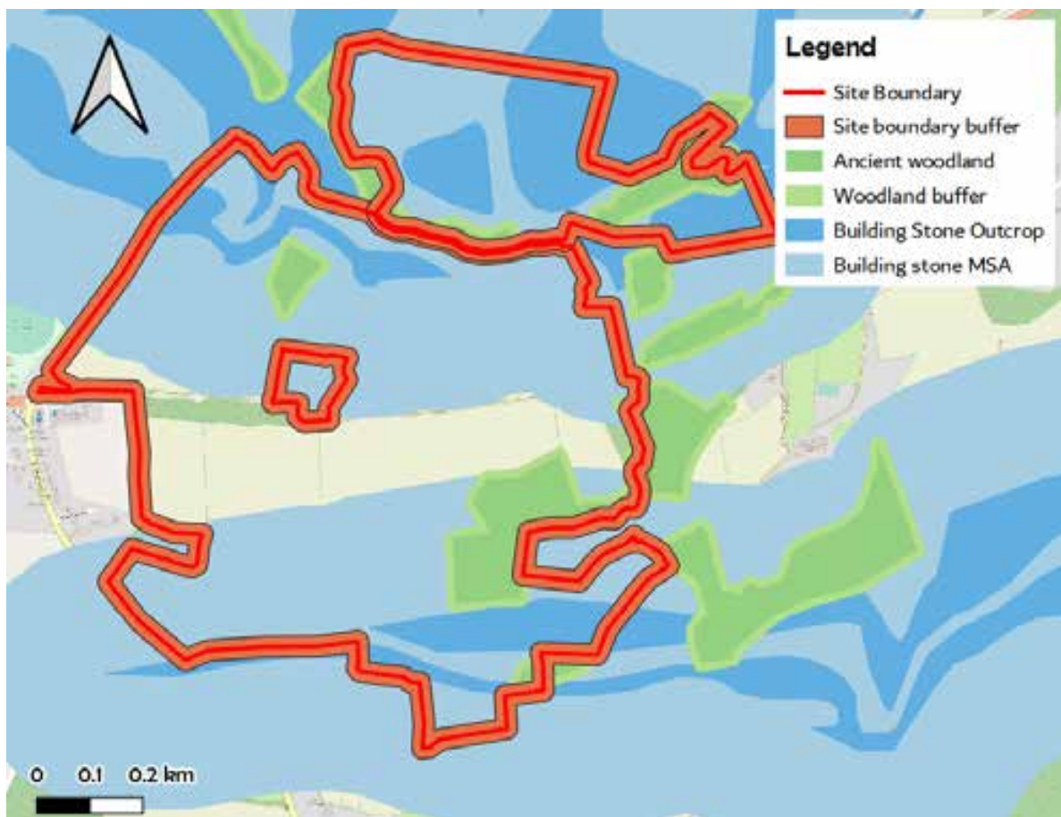
Figure 4-2 Building Stone MSA with buffer constraints
