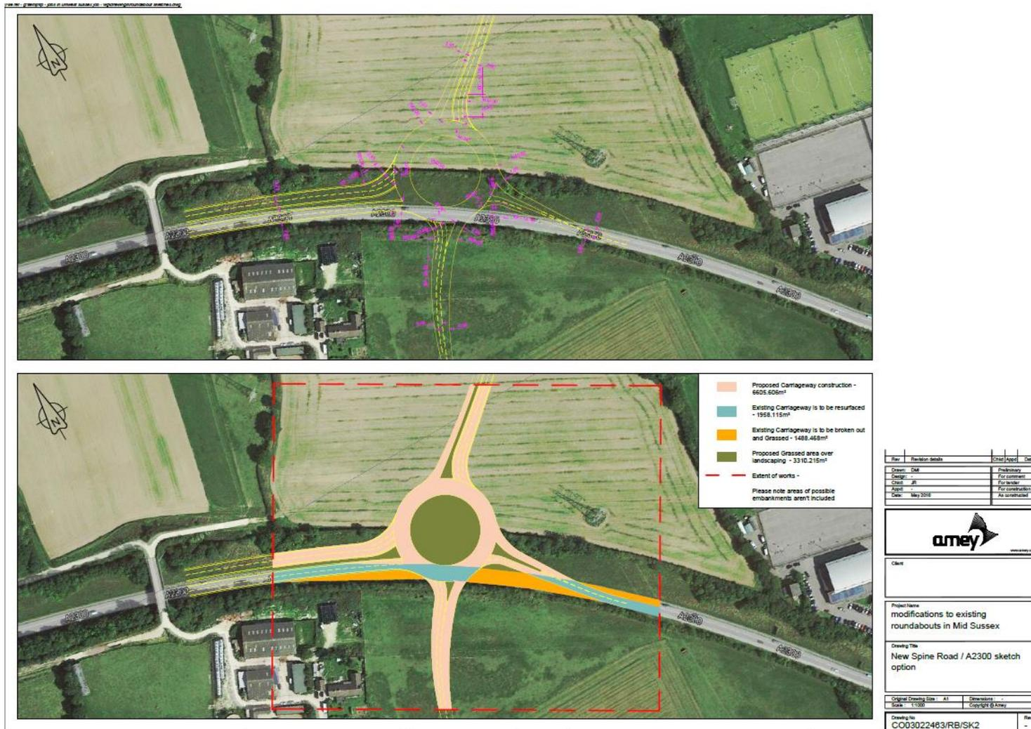
Figure 4: A2300/Northern Arc Spine Road (Proposed), Burgess Hill
