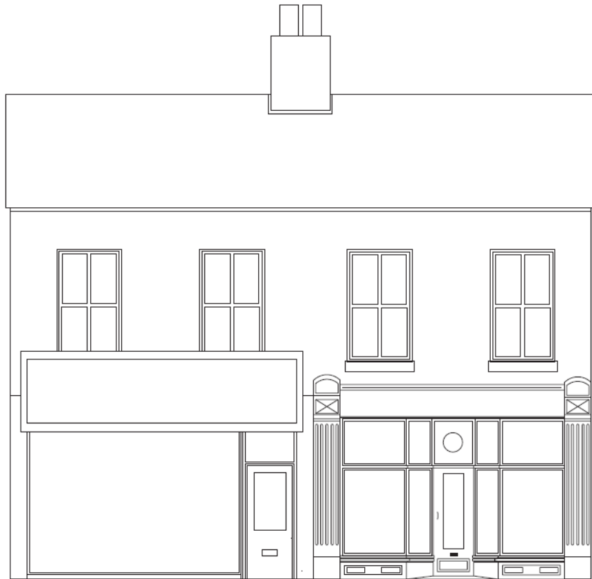
Modern, poorly-designed shopfront with excessive fascia
