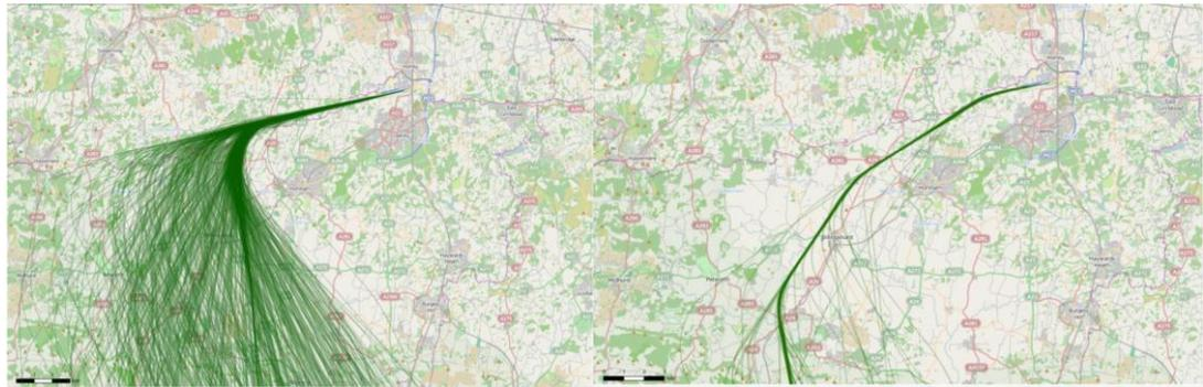
**FIGURE 5.1 ILLUSTRATION OF STANDARD DEPARTURE ROUTE (LEFT IMAGE) AND P-RNAV DEPARTURE ROUTE (RIGHT IMAGE) SWATHE WIDTH.**
