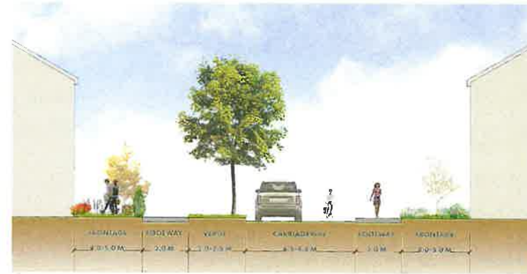
D THE LANES SECTION, WITH VERGE
